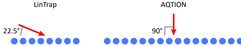
Figure 5.2: Single ion addressing geometry for the LinTrap setup (left) and the AQTION setup (right).
