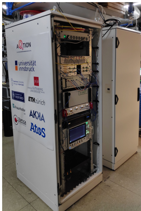
Figure 5.3: The AQTION setup is assembled in two 19-inch racks.
